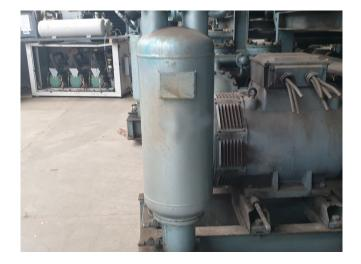
Manuel and Th VAN RUN UNITBOUW B.V. ROST 0 NEG- NR. 9005063 YEAR BUILT: 5.90 MEDIUM: R.22 CAPACITY: 0.056 m<sup>a</sup> DESIGN/TEST PRESS.22/38 BAR DESIGN TEMP.: 1.2 0 TYPE RO 100
